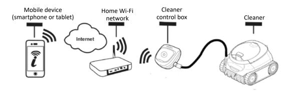
The iAquaLink™ app is available for iOS and Android systems: it provides additional functions. Use the iAquaLink™ app to benefit from advanced functions such as troubleshooting assistance by inputting error codes and have full control over the cleaner wherever you are, at all times.
